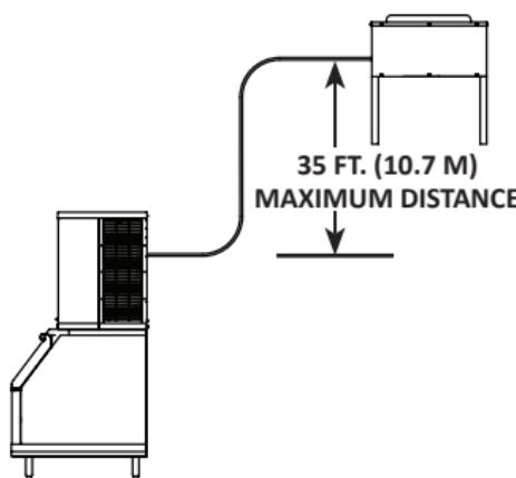
**35 ft. (10.7 m) Rise:** The maximum distance the Condenser or Condensing Unit can be above the ice machine.
